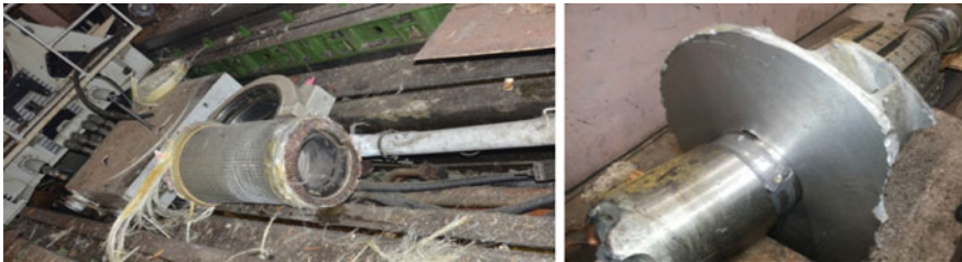
Fig. 1 Rotor assembly after failure at balancing tunnel for the failed rotor
