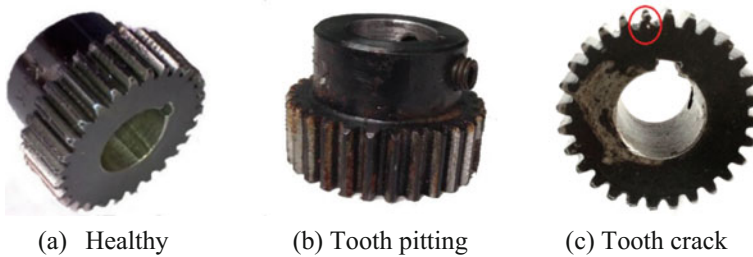
Fig. 3 The three considered health conditions of the sun gear
